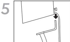
5 Place Airocide unit vertically onto the black pad atop the Stem, positioning the unit against the back mounting points.
