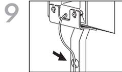
9 Snap power cord into the Cord Clips to hold cord in desired location.
