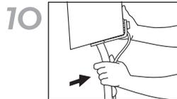
10 When moving the Floor Stand with the Airocide unit attached, lift the assembly from the stem and not the Airocide unit itself.
