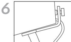
6 The mounting point should be between the Standoff Cylinders and the head of the Shoulder Bolts.
