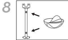
8 Peel the adhesive backing off of the Cord Clips and affix to the Stem in the location you desire.
