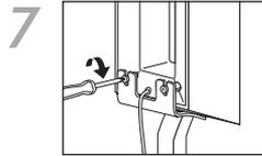
7 Tighten the Shoulder Bolts into the Airocide unit using a #2 Phillips head screwdriver.
