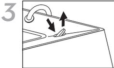
3 On the back of the Airocide unit, remove the 2 plugs closest to the power cord by pressing down on the exposed edge closest to the middle of the unit and then lifting the plug off by pulling on its outer exposed edge. Remove both plugs and save.
