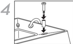
4 Slide Shoulder Bolts through the Standoff Cylinders and loosely hand-tighten them into the two lower bolt holes which were below the plugs. Leave about 1/4th of an inch between the Standoff Cylinders and the head of the shoulder bolt.
