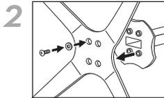
2 Affix Base to Stem by securing 4 Screw and Washer sets from the Base into the bottom of the Stem. Stand assembled Base upon a firm, flat surface.
